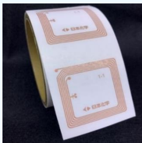
HF RFID antenna on paper
