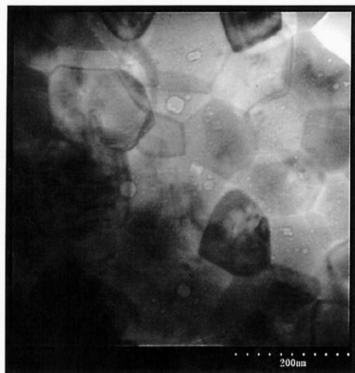
Fig. 12 TEM photographs of sintered hydrothermal barium titanate.
